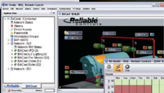
BACnet® System Panel Tree
